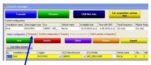
Activate "Channels" layer. It allows you setting the channels acquired by EVO3 and its layout depends on EVO3 version.
