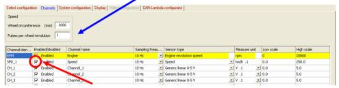
The figure below shows EVO3 Pro speed channels. Two of them are checked and the related boxes enabled, while the other two aren't.
