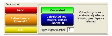
EVO3 can detect the engaged gear using an on-board gear sensor, sampling it from the ECU or calculating it using an algorithm based on engine RPM and Speed.
