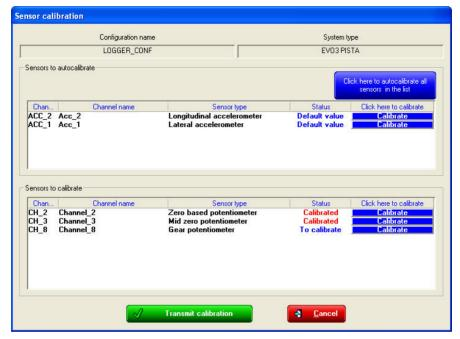
Transmit the configuration to the logger
